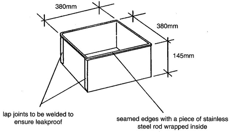
Overall dimension 380mm x 380mm x 145mm, to be made of a SWG 24 stainless steel (type 316) sheet. All edges should be seamed with a piece of stainless steel rod (dia. 5mm) to stiffen and avoid sharp edges. The lap joints should be welded to ensure that the whole tray is leakproof.
