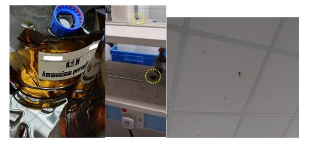
The photo on the left-hand side shows the Winchester bottle after the incident. Note that more than half of the bottle has disintegrated to produce glass projectiles. The next photo illustrates some small glass debris from the broken container found on the shelf near the bench where the bottle was stored. The last photo indicates glass debris embedded in the false ceiling.
