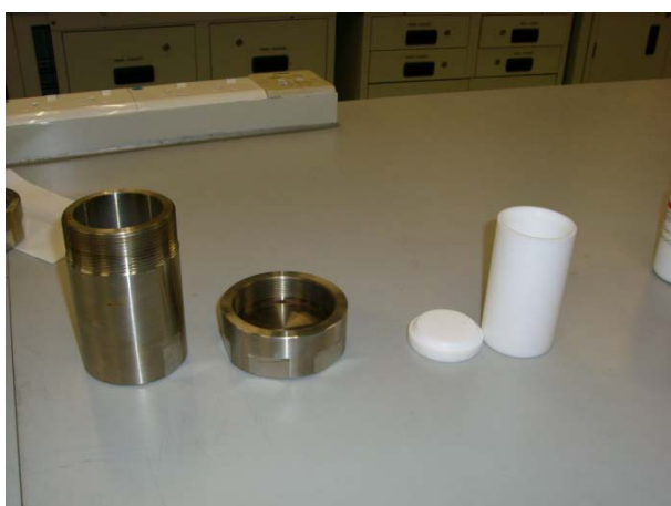
A vessel without safety device (similar to the one involved in the accident)
