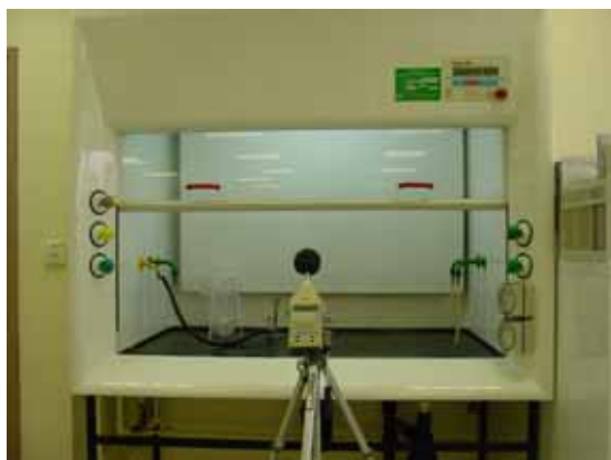
Figure 6: Measuring sound level generated by the fume cupboard.
