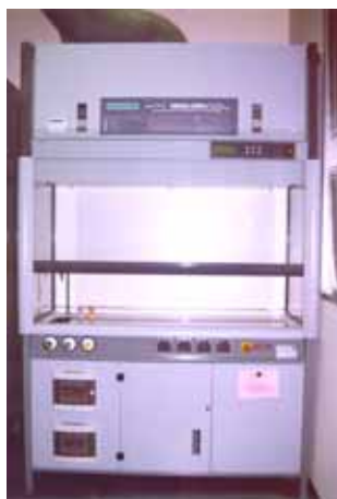
Figure 3: A re-circulatory fume cupboard with vortex scrubber and filters.
